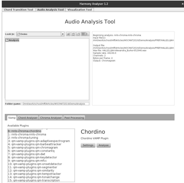
Fig. 6. Audio Analysis Tool from harmony-analyser.org : selecting a folder with WAV files and choosing a desired plugin for analysis (Vamp plugins, Chord Analyser, Chroma Analyser or Post Processing).
